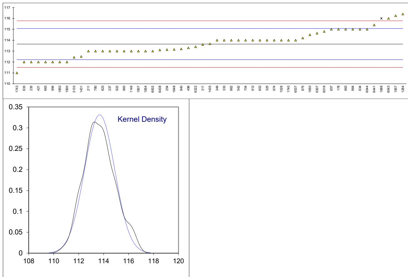
Determination of Kinematic Viscosity Houillon at 40 °C on sample #23082; results in mm<sup>2</sup>/s
