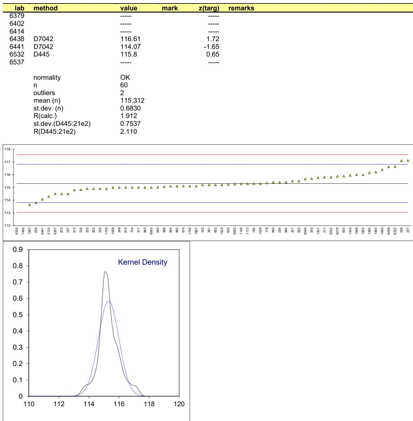
Determination of Kinematic Viscosity at 100 °C on sample #23082; results in mm<sup>2</sup>/s
