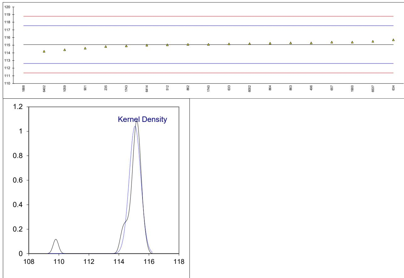
Determination of Kinematic Viscosity Houillon at 100 °C on sample #23082; results in mm<sup>2</sup>/s
